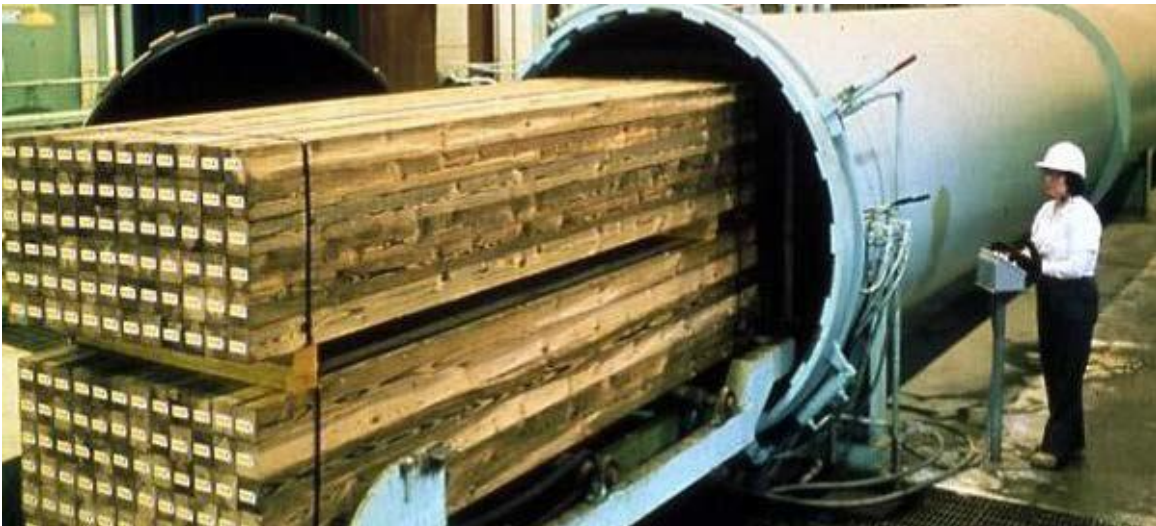
Wood being removed from a vessel following pressure treatment.
