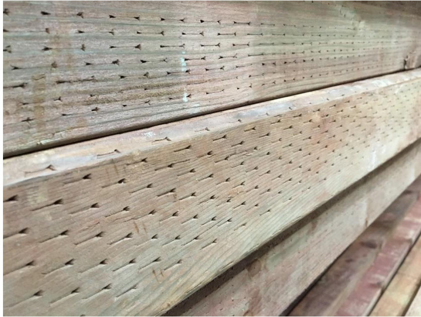
Example of pressure treated wood showing indentations from treatment.
